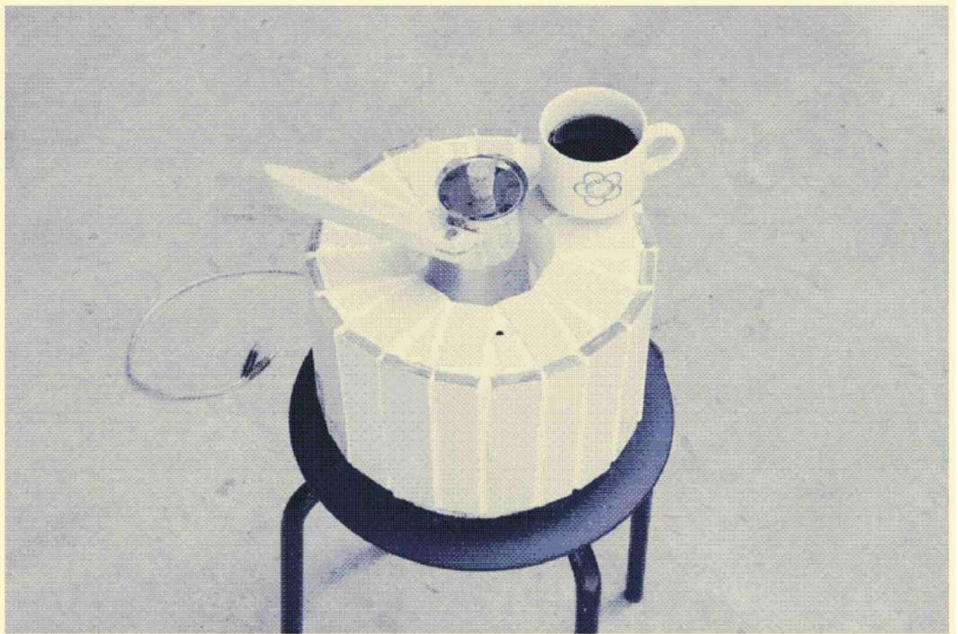
Image: The solar powered coffee maker that we build in this manual. Photo by Marie Verdeil. ☒
